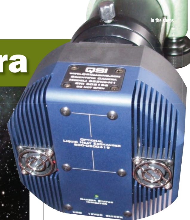
A rear view of the QSI 532 CCD camera showing the camera status indicator, cooling fins, twin low-inertia cooling fans, optional water cooling ports and USB and power connections.
