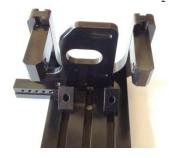
this, remove the risers and switch the sides then fully insert them. This will both point the tabs forward and will reduce the overall width of the risers. Next reverse the motor plate on its block and slide the focus motor assembly up between the tabs. Next slide the universal blocks up next to the other components. Next store the two 1/4-20 button head screws in the two threaded holes in
