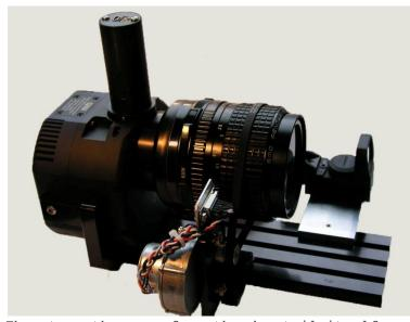
The strength comes from the dovetail itself, not the set screw. Please do not QSI583WSG with Lodestar guide camera mounted on QSI Dovetail Camera Mount, with Hurst focus motor, QSI 67 lens adapter, Pentax 67 55mm f/4 lens, prototype red dot finder plate, and red dot finder.
